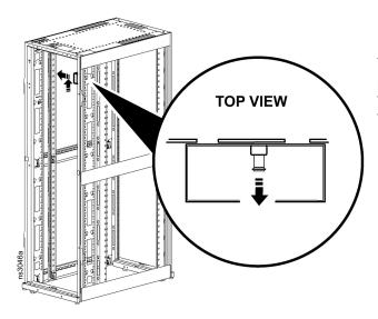
To remove the bracket from the rack, pull the plunger to release tension, lift the bracket up to the wider portion of the installation holes and pull the bracket away.
